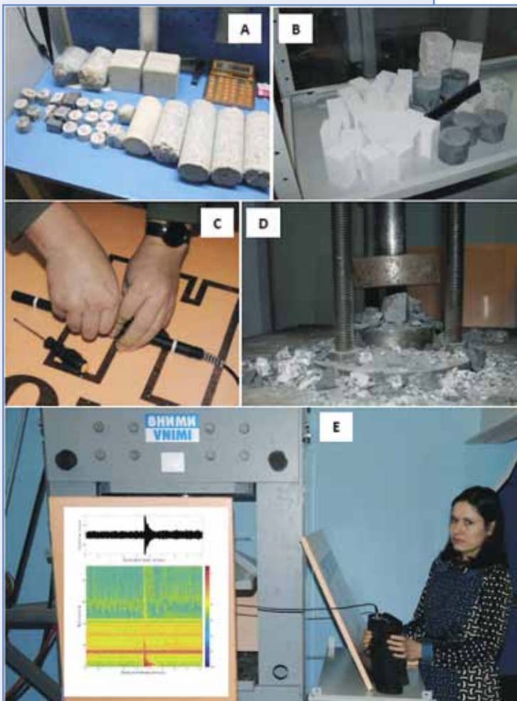
Fig. 3. An example of the visualization of field data obtained during the registration of EEMI (NER) in the mine workings of the Tashtagol field (VNIMI, 2017). The registered signal is at the top, the spectrogram is at the bottom
